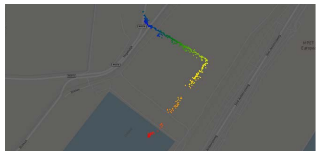
^^ ^^ Figure 1: 3D TDoA geolocations of a COTS DJI drone at one of the world's 15 largest ports. Red shows the most recent pattern of geolocations, while blue shows the oldest.
