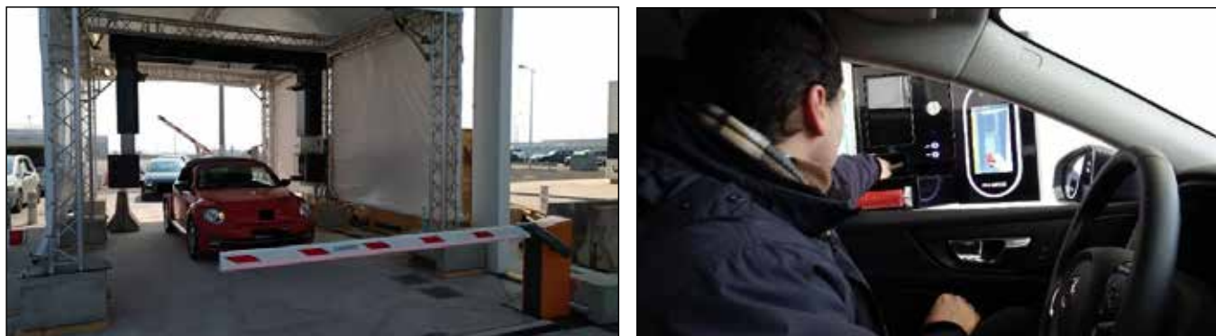
Figure 4. Car demonstration. Left image: Barrier behind the car closes the 'FastPass HdF' e-Gate. Right image: operating terminal (view from inside the car).
